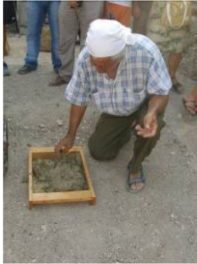
Mudbrick making process demonstrated by İsmail Cemal
