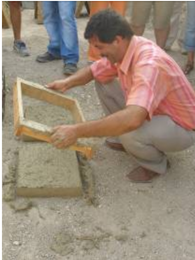
Trainees testing out mudbrick making
